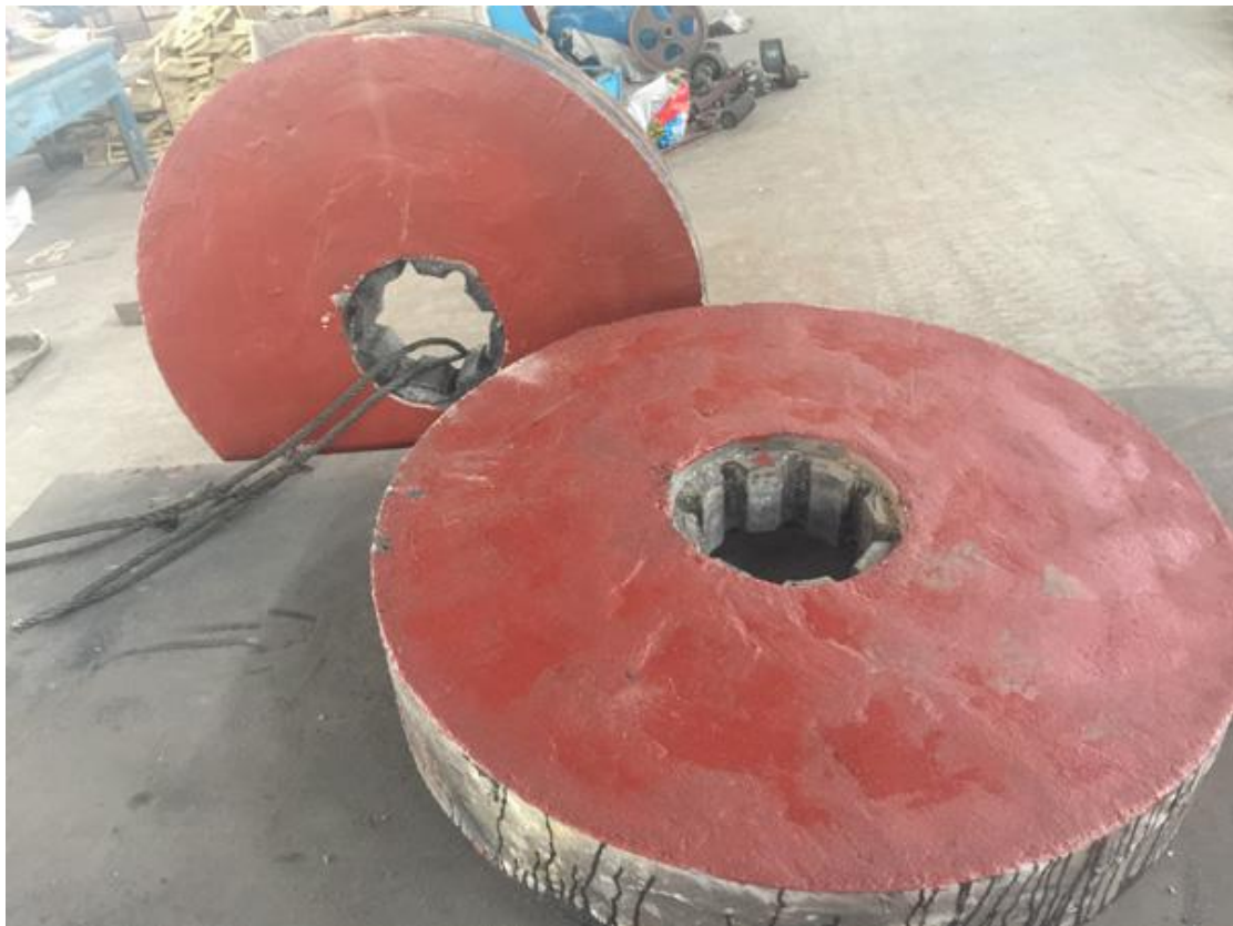
PAN MILL ROLLERS ( CASTING IRON MATERIAL, 1200MM DIAMETER, 200MM THICKNESS)
